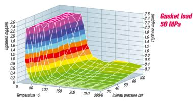
Tahtness mg/(sm) 2.0 1.8 1.8 1.6 1.4 1.2 0.8 0.6 0.8 0.4 -0.2 04 60 50 40 100 Internal pressure bar Temperature ° C
