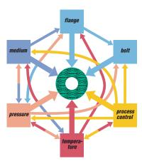
Maximum temperature and pressure values alone can not define a material's suitability for an application.
