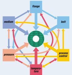
Maximum temperature and pressure values alone can not define a material's suitability for an application. These limits are dependent upon a multiplicity of factors as shown in the diagram opposite. It is always advisable to consider these factors when selecting a material for a given application.
